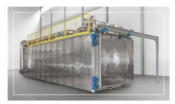
The best technology is used for the vacuum system: Liquid ring pump technology. The pumps have a long lifetime and are sized to provide a fast vacuum in safe conditions.
